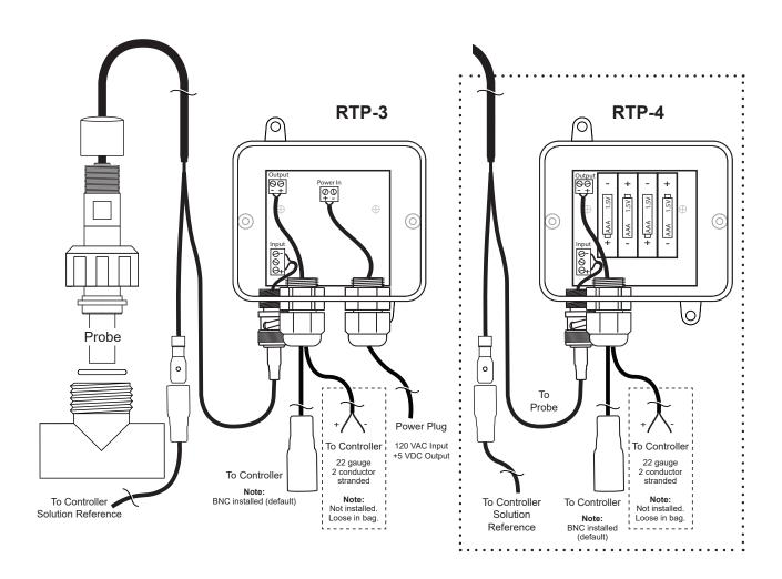
Pre-amps are supplied with both a BNC or twoconductor wire cable to connect between pre-amp and controller. The two-conductor cable can be ran directly to the pH input on the controller board. The BNC connector requires a special extension cable.
